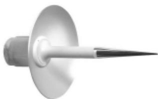
**Wile 253**, dishprobe for loose silage or hay. Measuring in a bucket (see 3.2.1 loose hay).
