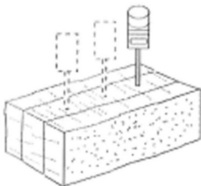
In smaller bales its enough to meaasure once but in bigger bales you need to have several measurements. Take the readings from different spots from the bale.
